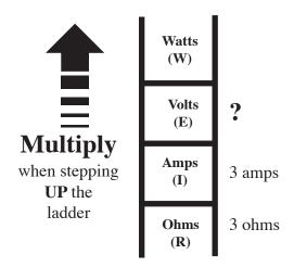
Solution: The "?" is above the numbers below, so you are going UP and you MULTIPLY, 3 ohms x 3 amps = 9 volts.
