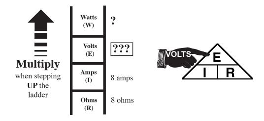
Solution: This question is requiring to skip a STEP (volts) to find watts with amps and ohms. With a ladder it is not safe to skip a step, so the first step is to find **volts** using the triangle.
