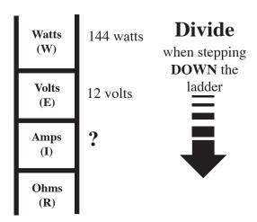
Solution: The "?" is below the numbers above, so you are going DOWN and you DIVIDE, 144 watts  $\div$  12 volts = **12 amps.**
