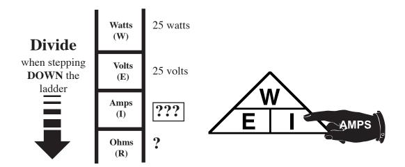
Solution: This question is requiring to skip a STEP (amps) to find ohms with watts and volts. With a ladder it is not safe to skip a step, so the first step is to find **amps** using the triangle.
