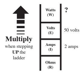
Solution: The "?" is on the top of the ladder with the numbers below, so you are going UP and you MULTIPLY, 50 volts x = 100 watts.
