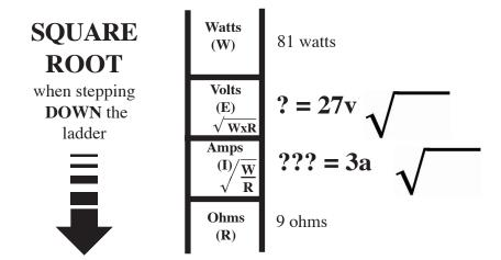
Solution: This question is requiring to step DOWN to find **voltage** with watts and ohms. Applying the squre root formula for volts which is 27 volts, but to make sure its the correct answer, you need to find the amps using the square root formula for amps and it is 3 amps.
