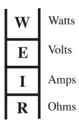
Then multiply the value below by the value above, stepping UP the ladder, or divide the value above by the value below stepping DOWN the ladder.
