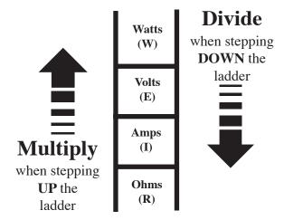
There's a simple alternative to using the Ohm's Law Wheel and trying to memorize all of those formulas. All you have to do is learn the elements of Ohm's Law; in the order above (top to bottom)....Watts (W) Volts (E) Amps (I) Ohms (R).
