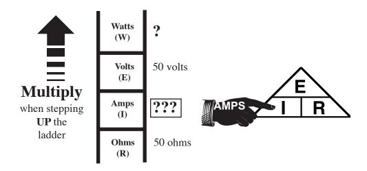
Solution: This question is requiring to skip a STEP (amps) to find watts with ohms and volts. With a ladder it is not safe to skip a step, so the first step is to find **amps** using the triangle.
