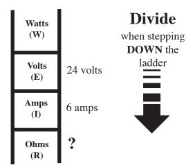
Solution: The "?" is on the bottom of the ladder with the numbers above, so you are going DOWN and you DIVIDE, 24 volts  $\div$  6 amps = **4 ohms.**
