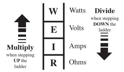
Example: What is the **resistance** in the circuit? The knowns are 24 volts and 6 amps. \_\_\_\_\_ ohms.
