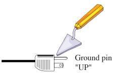
There is more chance of making contact with the top of a receptacle than the bottom as most receptacles are located 12-16" off the floor. A person stripping wallpaper is bringing the broadknife in a downward sweep towards the receptacle.
