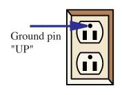
In my own experience, I have witnessed a painter stripping wallpaper with a broad-knife and as the broad-knife hit the receptacle the sparks flew when he made contact with the "hot" pin on the plug on the cord to his fan. If the grounding pin had been installed in the "UP" position, the broad-knife would have come into contact with the grounding pin rather than an energized pin.
